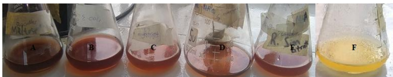
Plate 1. Discoloration of supernatants of bacterial cultures due to AgNO 3 reduction. A = Bacillus -synthesized AgNPs; B = E. coli -synthesized AgNPs; C = Micrococcus -synthesized AgNPs; D = Staphylococcus aureus -synthesized AgNPs; E = Pseudomonas aeruginosa synthesized-AgNPs and F = Control.
